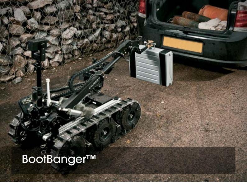
The BootBanger™ is an innovative IED extractor / disruptor used primarily against Vehicle-Borne Improvised Explosive Devices (VBIED). Intended for extracting IED main charges from the load carrying area of a car.
