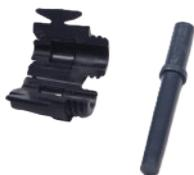
The Split Screw™ used in conjunction with the PDA provides an effective way of securing the detonator into the charge without risk of the detonator becoming loose or falling out (detonator not included). The Dummy Detonator allows you to set up the charge to ensure the explosive can accommodate the detonator effectively. The dummy detonator is replaced with a live detonator when ready.
