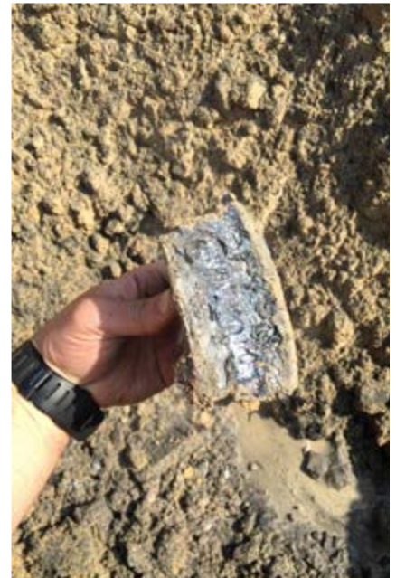
Cutting Steel: NX3600 charge used, 45mm severed
