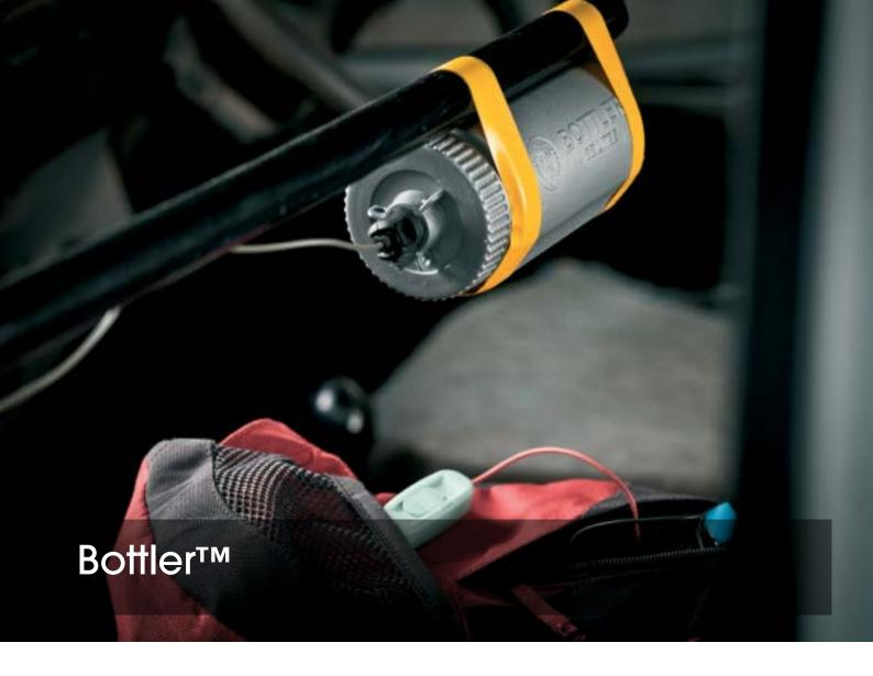
The Bottlers<sup>™</sup> constitutes a family of small to medium sized omnidirectional Improvised Explosive Devices (IED) disruptors. Additionally they can be used to burst open vehicles or other containers defeating IEDs within them.
