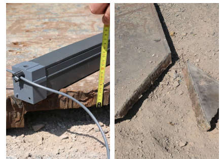
Applied to 50mm steel - before & after
