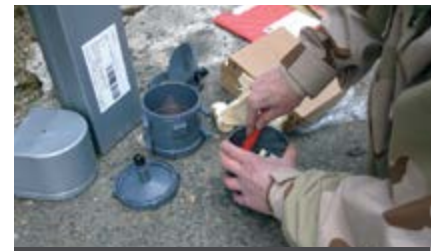
Loading Krakatoa™ with Explosive
